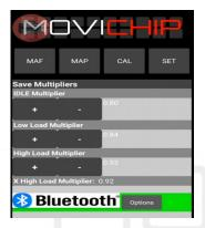
If the load signal is over 20% and less than 60%, the MAF Manager will use the "Low Load Multiplier".
