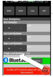
This is an auxiliary multiplier which may be used with the auto tune function, if the auto tune function deems it necessary. If, after a session this multiplier is different from the high load multiplier it suggests your MAF sensor is going out of range. If your MAF sensor is going out of range you should change to a MAF sensor that can measure the full range of air flow through the engine.
