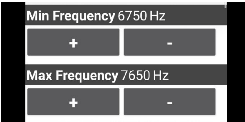
Figure 10 - Setting the knock frequency window to be monitored
